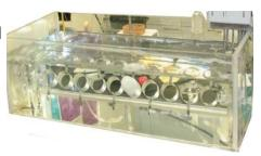
9200.1-86 estimates the oral bioaccessibility of both lead and arsenic from soil by simulating the stomach fluid of a swine. The analysis is highly controlled in terms of temperature as well as pH of the fluid.
